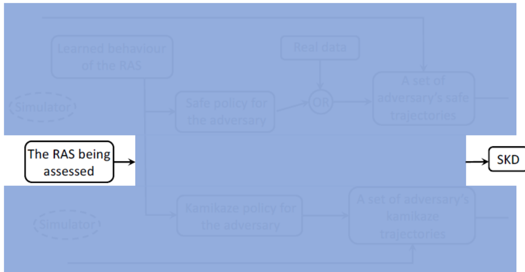
Figure 3 - Consumers can view the mechanism shown in Figure 1 as a black box. The greyed area does not need to be revealed to the consumer.
